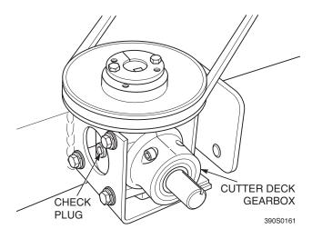
Figure 7-9. Cutter Deck Gearbox
